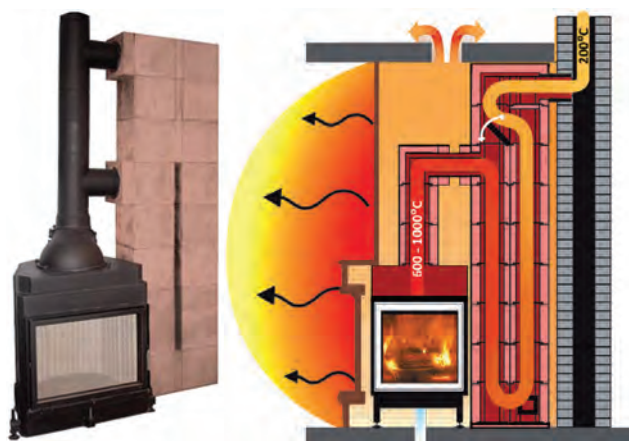
Fig. 1. The tiled fireplace – the appearance and the diagram of operation [8]
