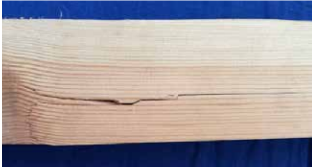
Fig. 3. Typical failure mode of reference beams
