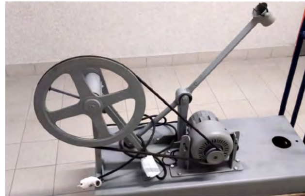
Fig. 2. Device for mechanical mixing of samples during testing of grouts using the foam index method
