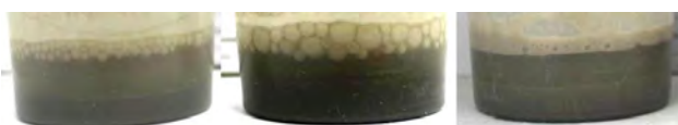
Fig. 1. Stable foam on the surface of cement grout samples, with various superplasticizers
