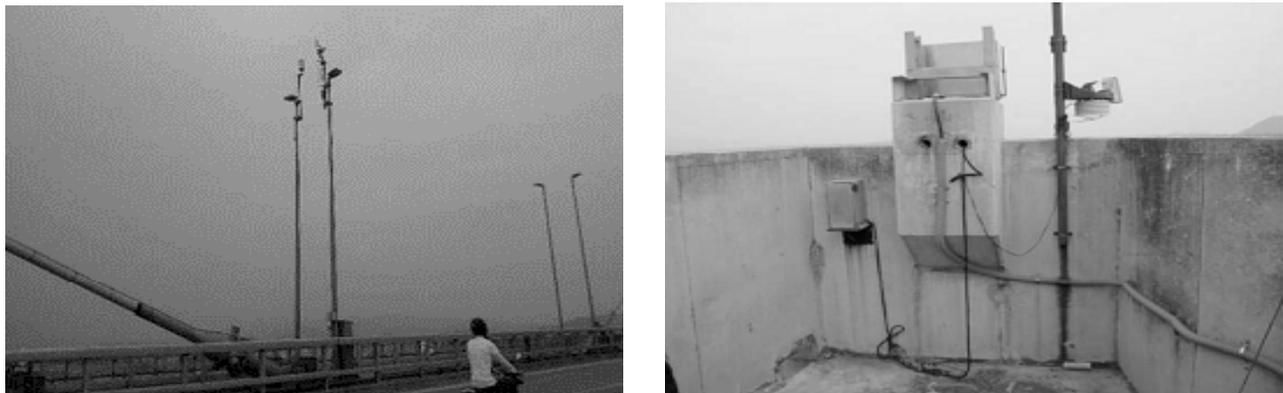
Fig. 2. Weather station install in main desk and on the top of pylon anchor of Bai Chay Bridge
