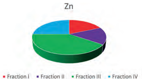
Fig. 8. Average percentage share of zinc in sludge from the Daleszyce sewage treatment plant depending on the fraction
