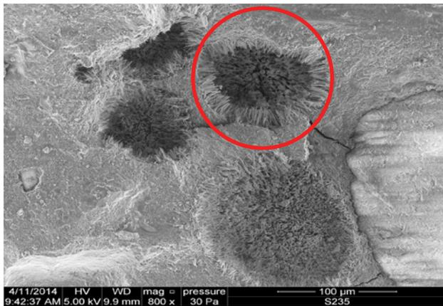
Fig. 4. Microstructure of AE OPC mortar immersed for 64 weeks in the solution of 5%  $\text{Na}_2\text{SO}_4$  (SEM 800x). The mean expansion of specimens was 5.9%. ( $\text{C}_3\text{A} = 6.3\%$ )
