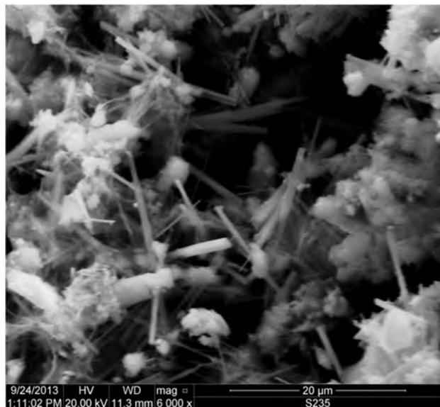
Fig. 2. Microstructure of nAE OPC mortar immersed in the solution of 5%  $Na_2SO_4$  for 64 weeks (SEM 6000x). The mean expansion of specimen was 5.7%. ( $C_3A = 6.3\%$ )
