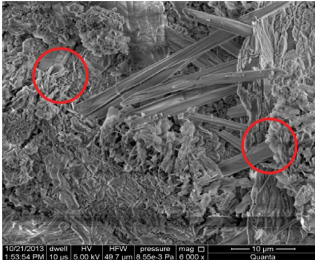
Fig. 1. Microstructure of nAE OPC mortar immersed in the solution of 5%  $Na_2SO_4$  for 12 weeks (SEM 6000x). The mean expansion of specimen was 4.6%. ( $C_3A = 11.5\%$ )
