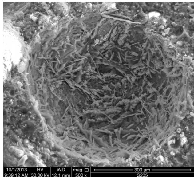
Fig. 3. Microstructure of AE OPC mortar immersed in the solution of 5%  $Na_2SO_4$  for 12 weeks (SEM 500x). The mean expansion of specimens was 8.8%. ( $C_3A = 11.5\%$ )
