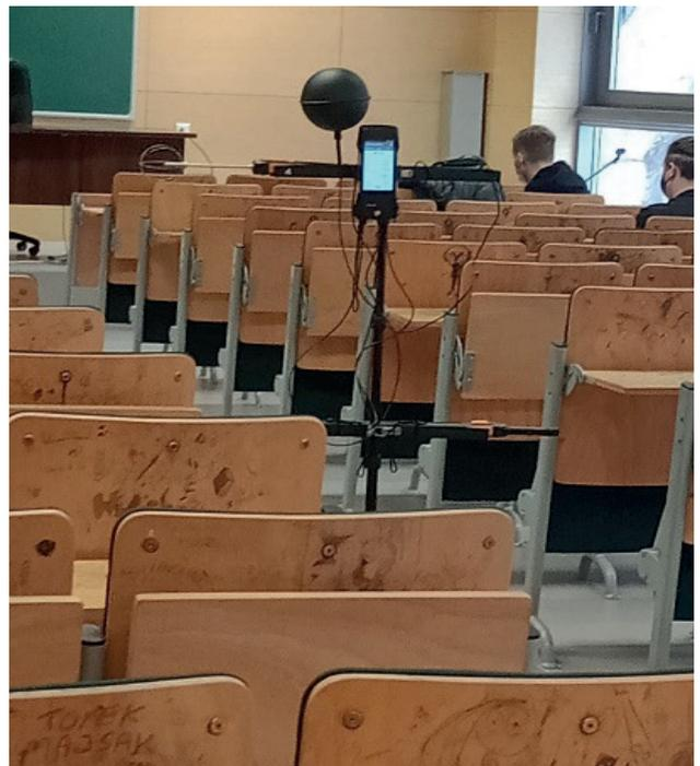
Fig. 2. Microclimate meter with the probes
