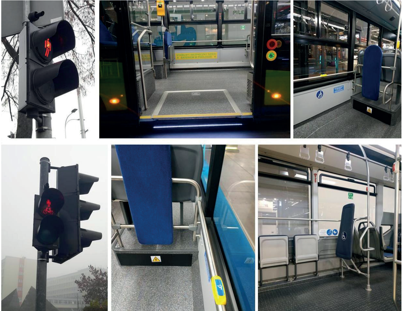
Fig. 8. Senior-friendly elements when traveling by public transport: light and sound signaling at crossings, stable and safe bus passage thanks to batteries in the floor, comfortable space for wheelchairs, seats, handrails, buttons – dedicated to seniors. Photo: Joanna Gil-Mastalerczyk
