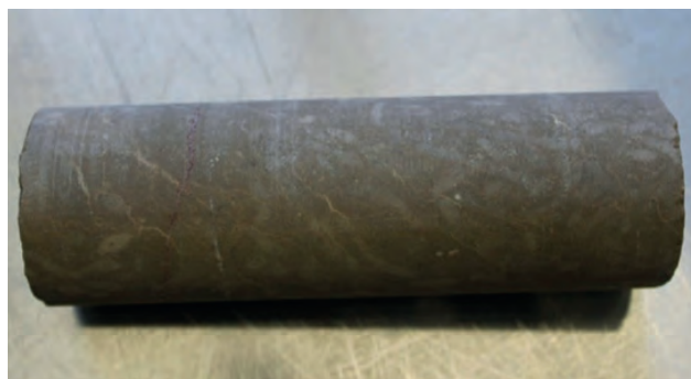
Figure 1. DAVS test specimens with dimensions \phi 50 and h = 150 mm [own elaboration]
