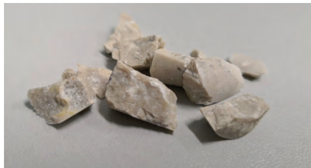
Figure 2. Samples prepared for MIP testing [own elaboration]
