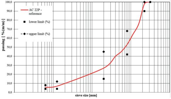
Fig. 2. Mineral mixture grain size curve
