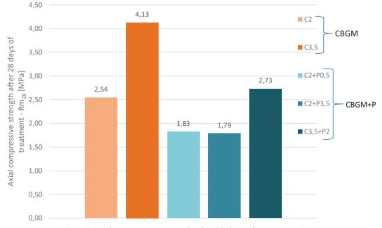
Fig. 6. Axial compressive strength after 28 days of treatment –  $Rm_{28}$
