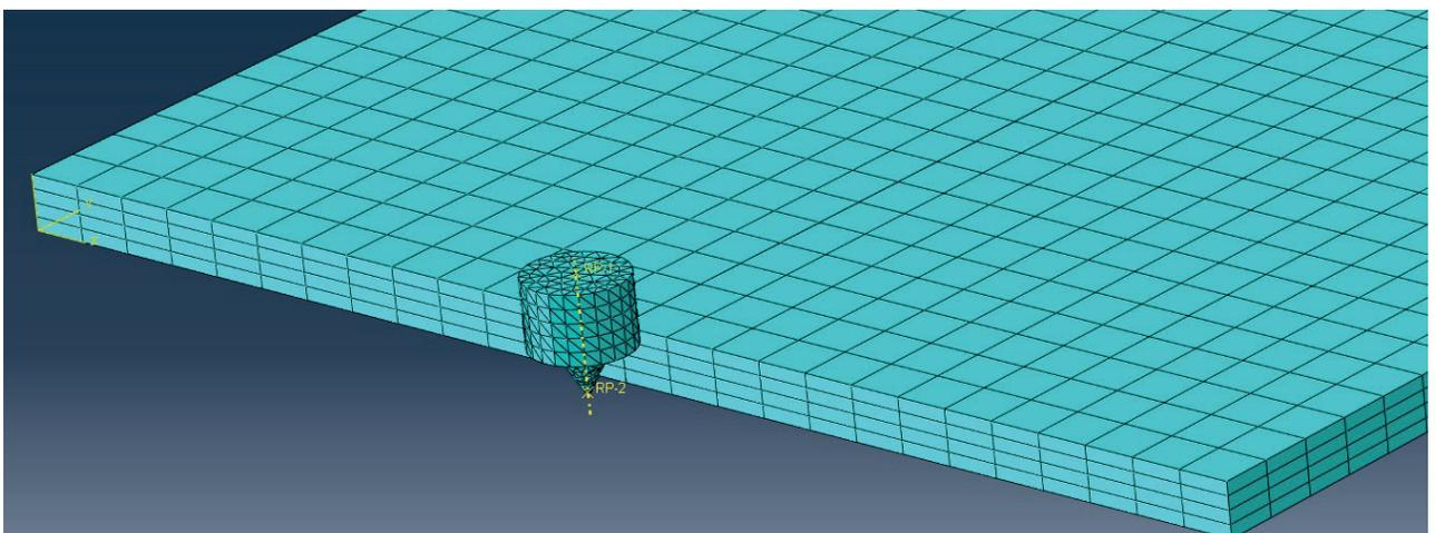
Fig. 6. The magnified welding tool with the edges of the plates
