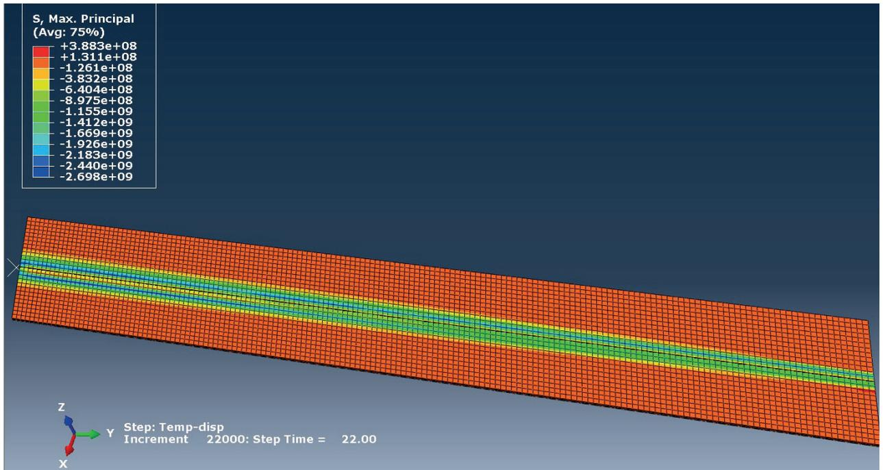
Fig. 10. Maximal principal stress after time  $t = 22.0$  s; all results expressed in Pa
