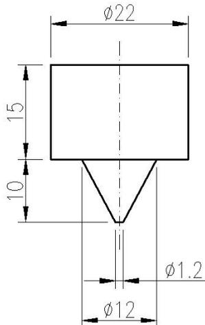
Fig. 4. Geometry of the welding tool (dimensions in [mm])
