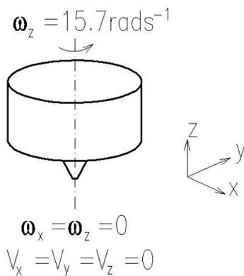
Fig. 9. Boundary conditions – angular velocity of the welding tool
