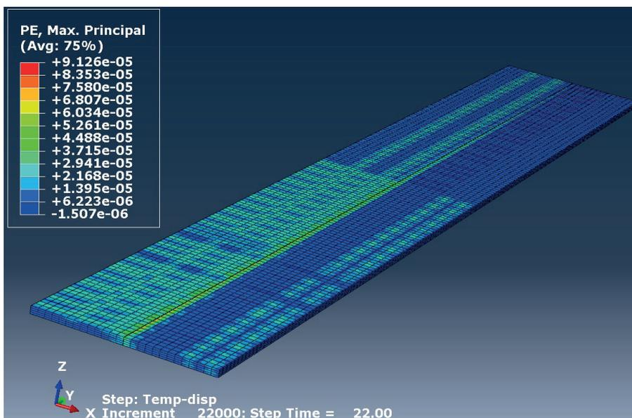
Fig. 16. Maximal principal plastic strains after time  $t = 22.0$  s
