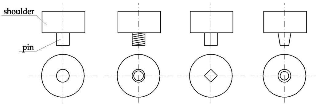
Fig. 1. Sample shapes of the operating tool used in the FSW process
