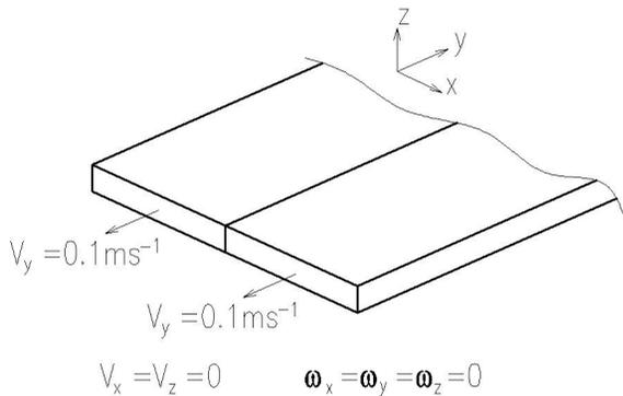
Fig. 8. Boundary conditions – transverse velocity of the welded plate
