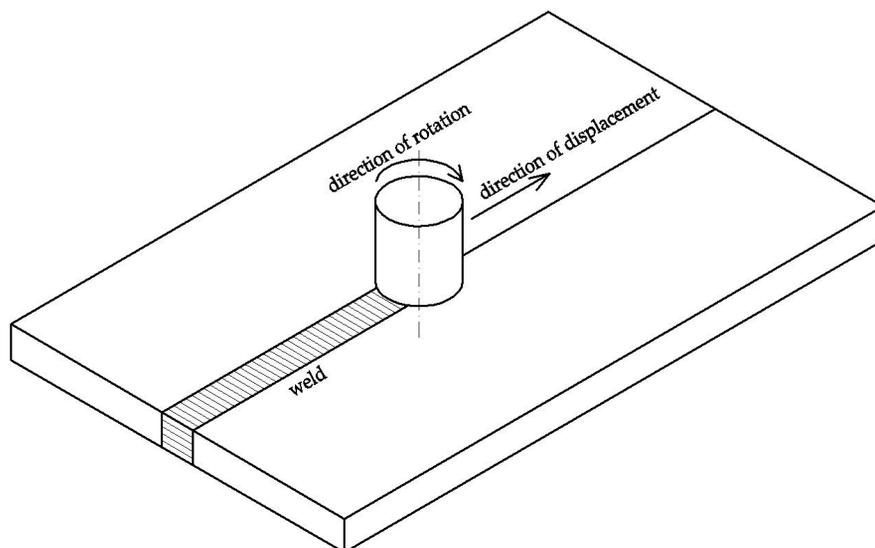
Fig. 2. General view of the FSW process
