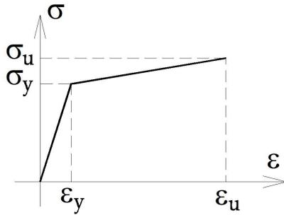
Fig. 7. Stress-strain curve defined in the numerical model
