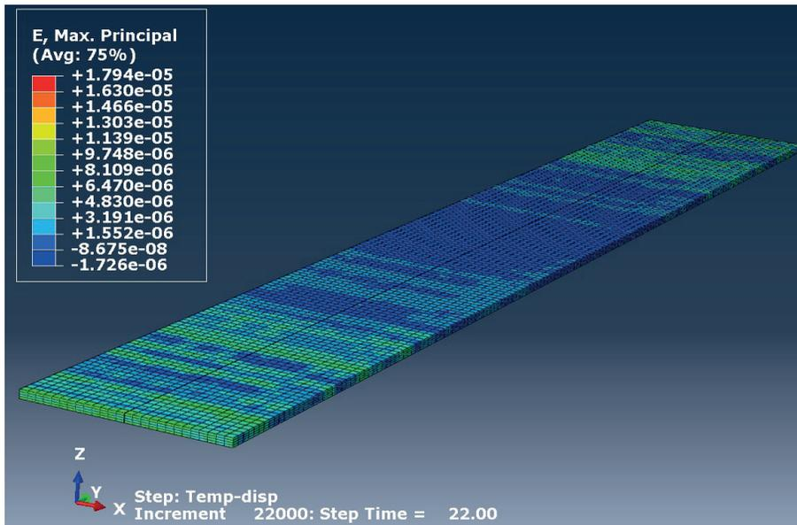
Fig. 15. Maximal principal total strains after time  $t = 22.0$  s
