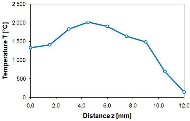
Fig. 13. Nodal temperature in a transverse section of the right-hand side plate vs distance z from the top of the plate,  $t = 11.0$  s
