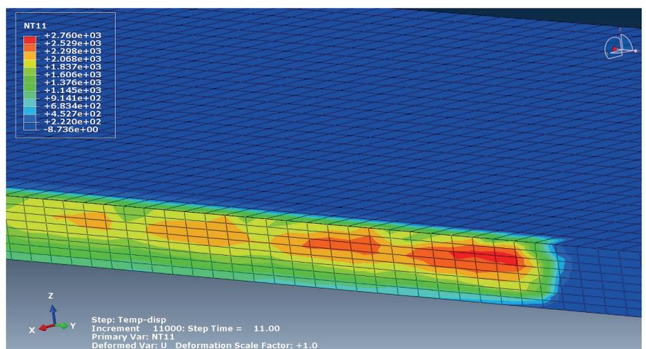
Fig. 12. Nodal temperatures (in °C) in a longitudinal cross section of the weld,  $t = 11.0$  s
