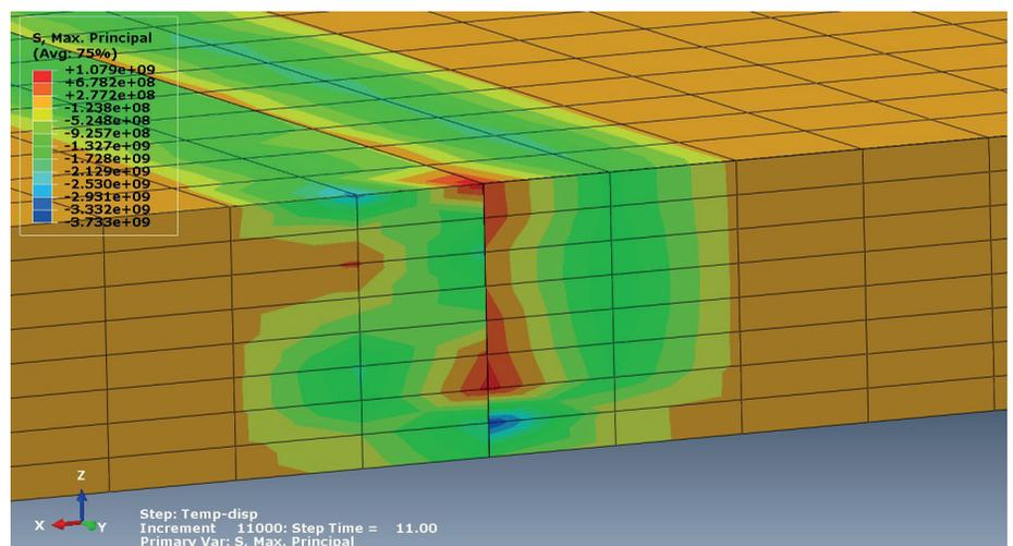
Fig. 11. Maximal principal stress in a transverse cross section of the plates,  $t = 11.0$  s
