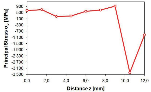
Fig. 14. Principal stress in a transverse section of the right-hand side plate vs distance z from the top of the plate,  $t = 11.0$  s
