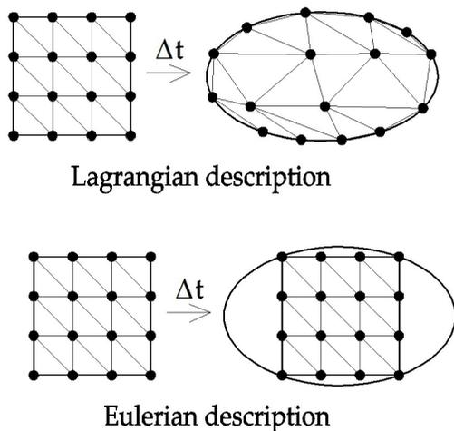
Fig. 3. Different mesh behavior in the Lagrangian and Eulerian formulation
