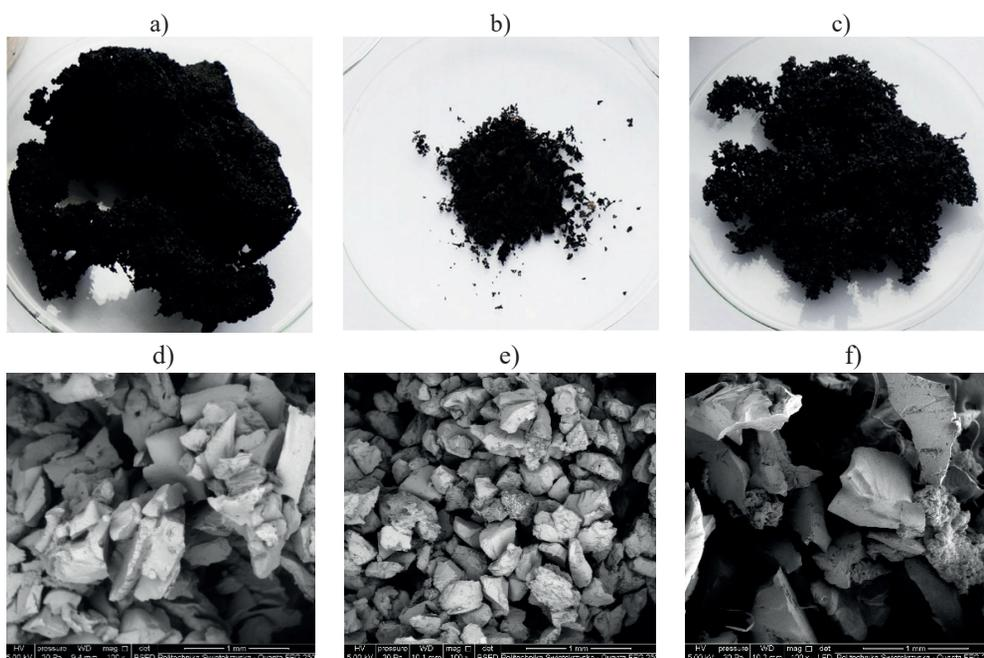
Fig. 2. Images of the rubber crumbs recovered from the selected joint sealants: a), b), c) MS3, MS5, MS6 – without magnification; d), e), f) MS3, MS5, MS6 – magnification × 100 by scanning electron microscope
