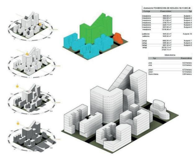
Fig. 2. Compilation of apartment areas for an example building mass with sunlight and shading analysis
