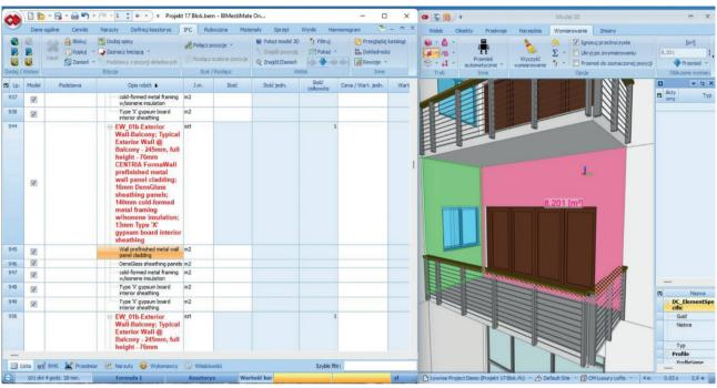
Fig. 5. Automatic creation of the scope of work in the BIMestiMate program along with quick quantity calculations "by indication" of the element and selection of the unit of measure (source: own elaboration)
