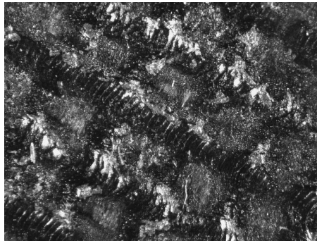
Fig. 3.7. Stereoscopic photographs of the laser-treated Cu-Mo surfaces (x40 magnification)
