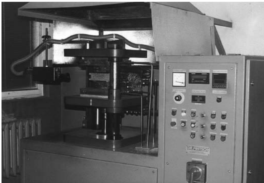
Fig. 2.6. Hot pressing operation carried out in air [22]
