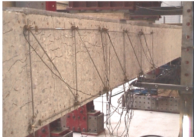
Fig. 6. Shear tests on beams damaged by many horizontal cracks due to Alkali Silica Reaction (TU Delft)
