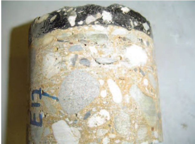
Fig. 5. Drilled cylinder with visual flaw under one of the large particles (weakened interface)
